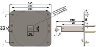
Ballast gravel pan for solar collectors on tilted frames on flat-roof.
