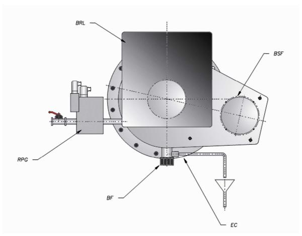
Figure 4181.01: Condensate connection
