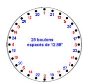
Figures showing the tightening sequence to comply with
