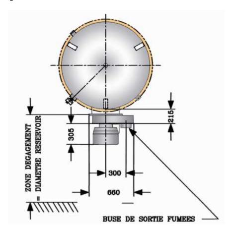
Figure No. 3123.12: Indicative figure showing the Burner / Heat exchanger dimensions
